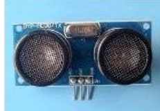
26580631 DYP-ME007TX Ultrasonic sensors 3pin (serial port output way) ///
