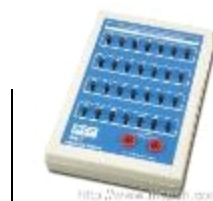
23706010 Boitier decade INDUCTANCE MATRIX,Range: 0~ 111.1mH(10?H steps) with 4decades, Accuracy : 5%,Current limit: 100mA,Internal stray inductor:0.6?H
