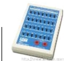
23706010 Boitier decade INDUCTANCE MATRIX,Range: 0~ 111.1mH(10?H steps) with 4decades, Accuracy : 5%,Current limit: 100mA,Internal stray inductor:0.6?H
