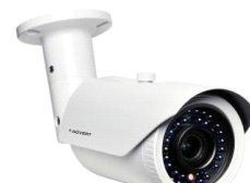
29705786 1/3' APTINA Sensor, 1.3Megapixel, Resolution 1280*960PP, 2.8~12mm Megapixel lens with ICR, 42pcs Oblong IR Leds, Support Admin Vision
